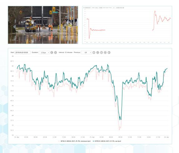
Being able to capture system transients within the water distribution system allows operational teams the ability to review the impacts of operational decisions – both occurring within the distribution system infrastructure and from the associated pump stations.
