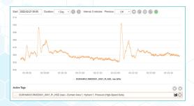
As part of this project, the Region has also integrated their SCADA data into the hydrant. All platform and are now able to directly see the impact of operations on the pressures and transients in their network. This has enabled the Region to identify transients through alerts and trace their causes all in one place, reducing effort while allowing for more in-depth and timely investigations.
